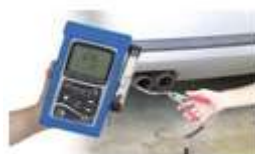
FIG 5: Exhaust gas Analyzer
